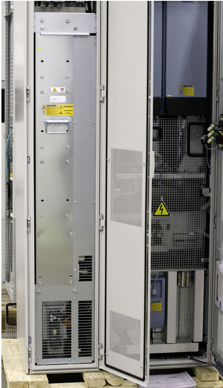
Figure 72. An LCL filter
